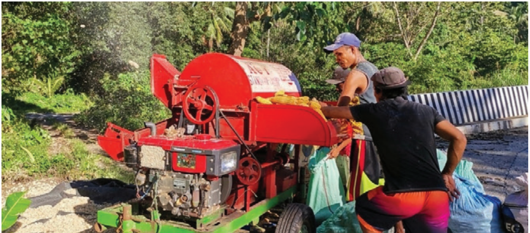
The group attests the machinery made harvesting process easier than manual operations because the machine separates grains from the rice straw.
