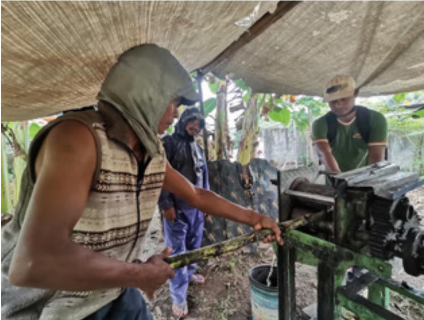
Members of KFA on showing how to extract sugarcane juice using the presser provided by the SAAD program.
